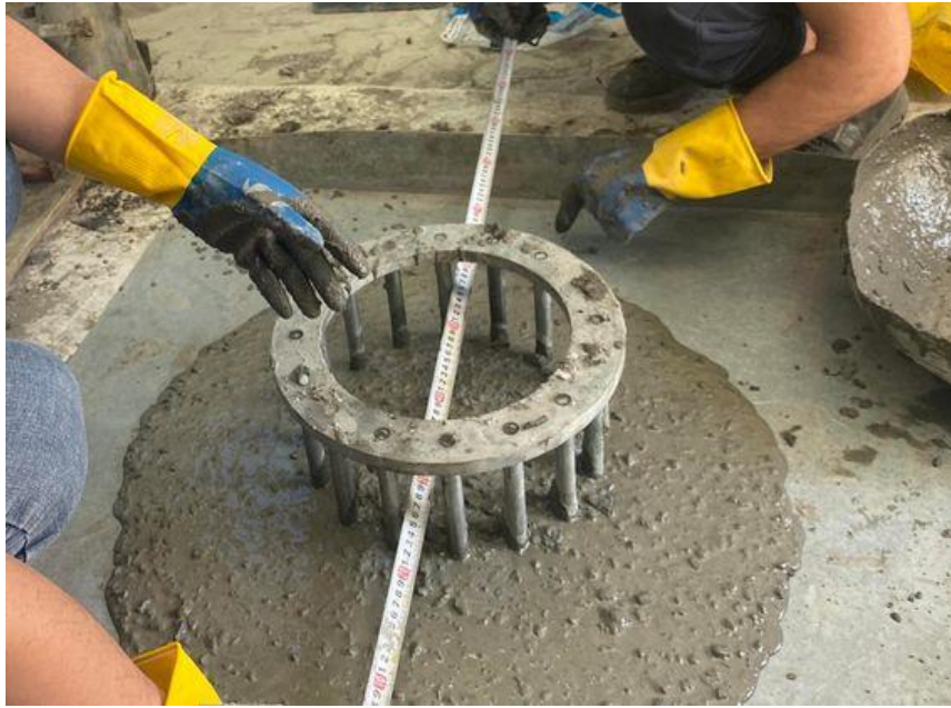
J-Ring test instruments and procedure
