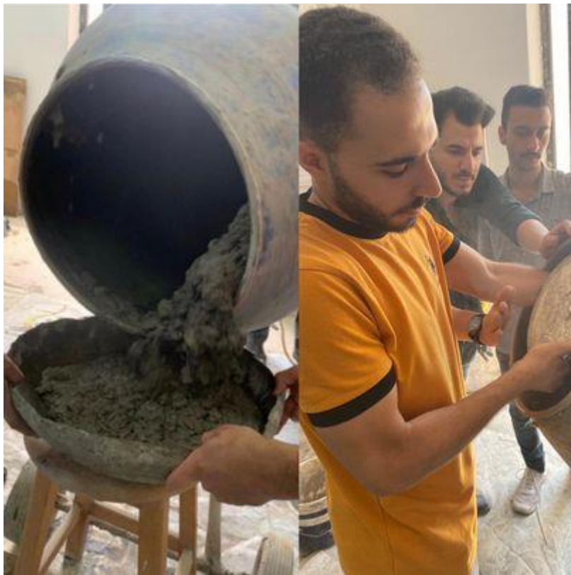
Concrete mixing in a batch drum mixer
