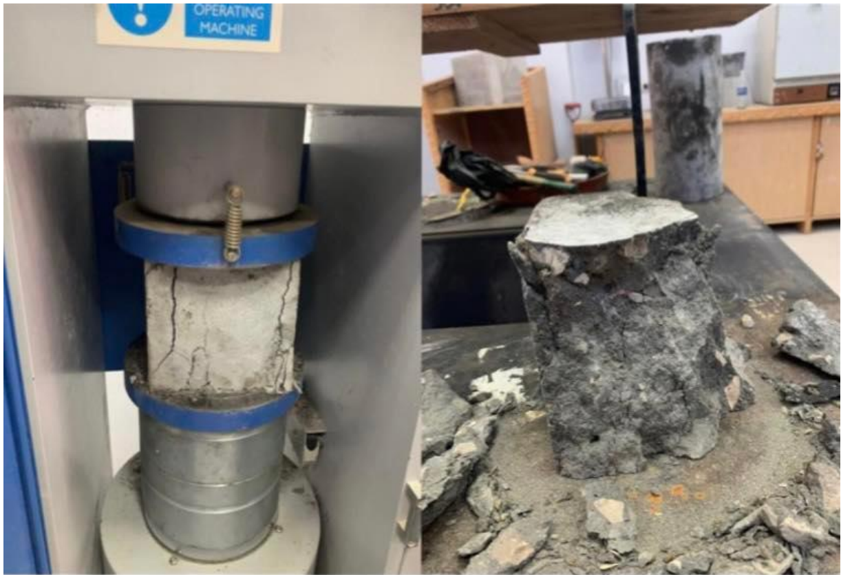
(A) Cube compression test at failure (b)
