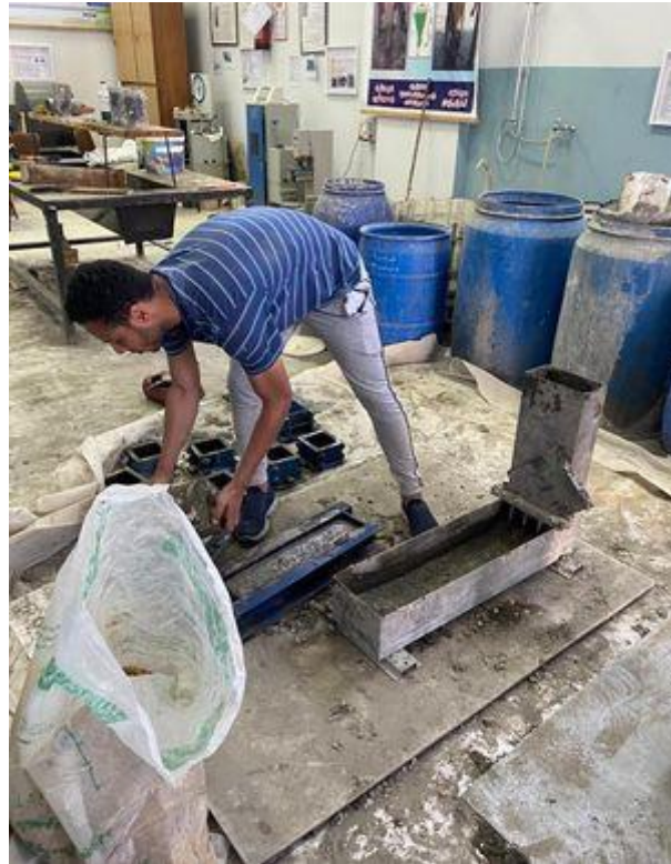
Casting and compaction
