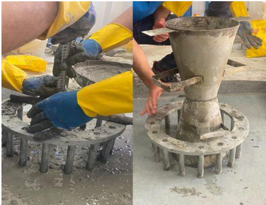
J-Ring test instruments and procedure
